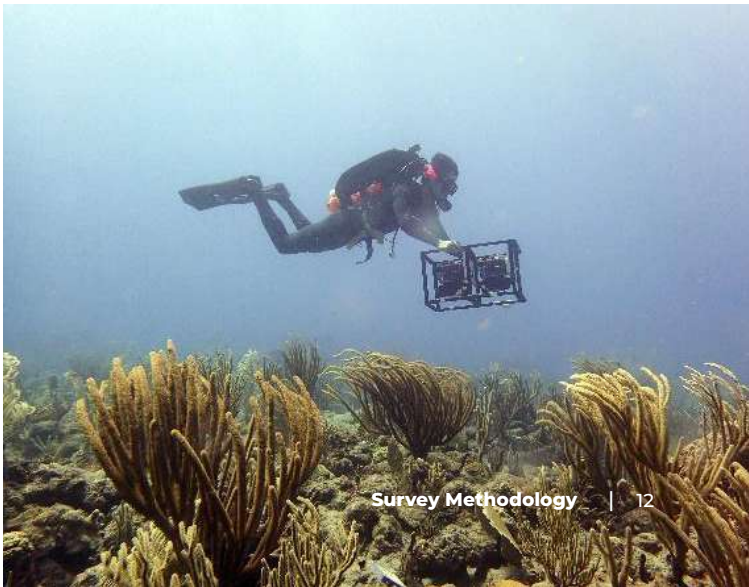
FIGURE 2: Photomosaic data collection method. Each photomosaic is stitched together from ~2000 photos acquired by swimming back and forth over the reef in the pattern on the left.
